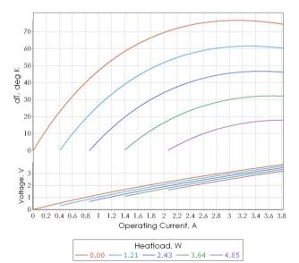
**Note**: Performance data is specified at optimal optimal conditions (TEC hot side is stabilized at ambient temperature). Heatsink thermal resistance is not included into estimations. Use TECCad Software for estimations under different conditions.
